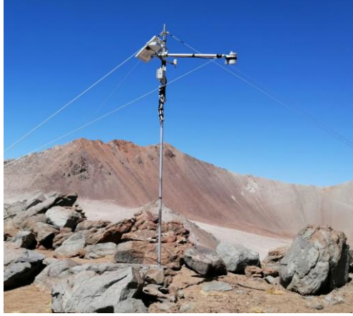
Fig.2 Prototype node implemented in 2021 summer season near Tascadero AWS
